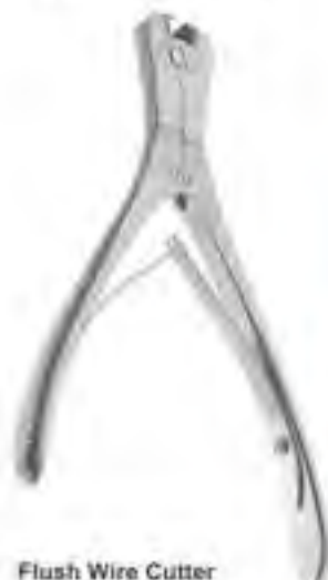
Flush Wire Cutter 10-1216 17cm Front and side cutting w/ carbide inserts, double action. Max capacity, 1.5mm
